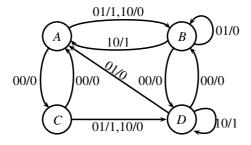
The circuit has two inputs  $(x_1, x_0)$  and one output (z). The inputs can take the values 00, 01 and 10 (the value 11 will never occur and can be considered as a don't care).
