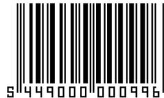
The most spread code which tends to become a standard is the EAN-13. This code is formed by 13 digits: the 12 first correspond to the code of the product, and the last one is a digit of control. The digit of control is a very important part of the EAN coding, because it makes possible the elimination of the reading errors.
