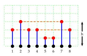
Since wires must not overlap, some care must be taken to decide the level of each horizontal connexion. Note that vertical connexions are not a problem because they can never overlap. Please compute the minimum number of levels h needed to connect all the pins with no overlaps. In the example, it is impossible to connect the four pins with less than three levels.
